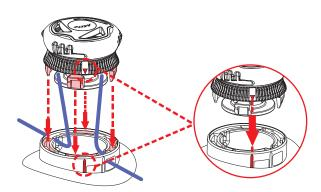
2. Turn the knob on the counterclockwise, and ensure that the arrow on the top knob and the one on the base are aligned. After you hear the "Click" sound, this means that the procedure is done.
