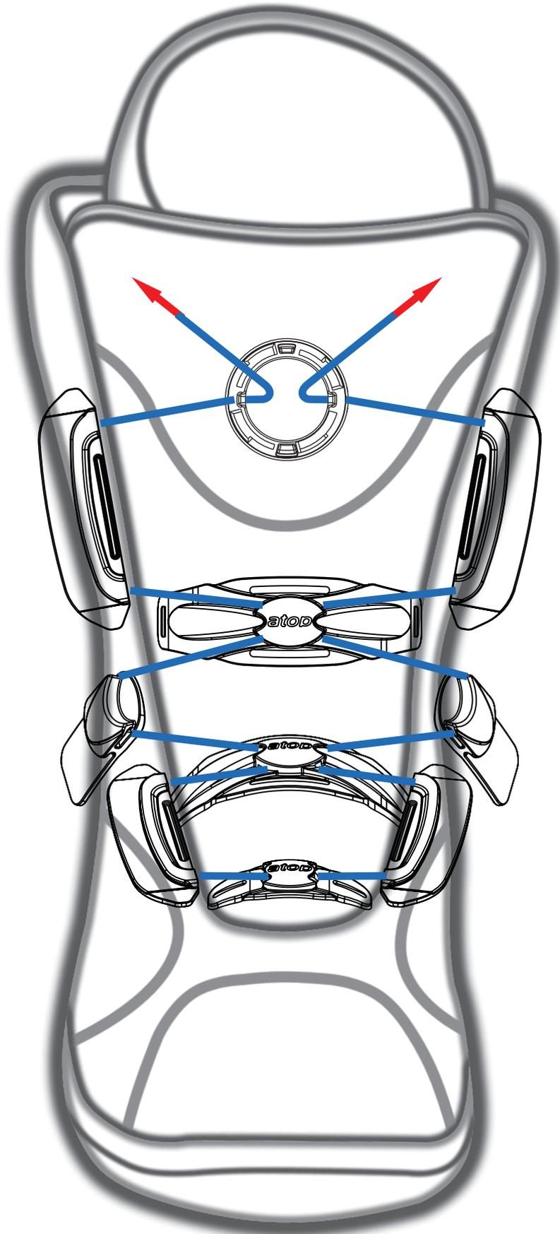
2. Turn the knob and align the arrows to any of the four hooks.
