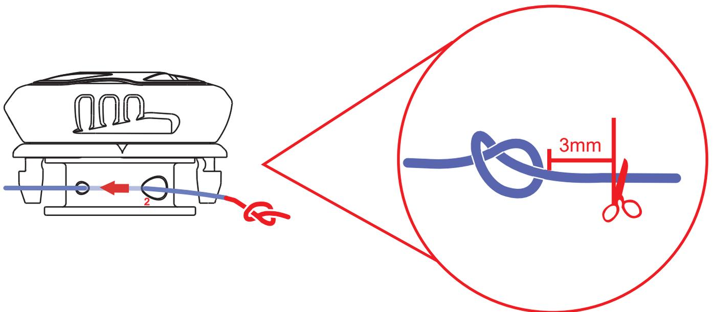
( 4 ) Thread wire's terminal back to hole 2 to the bottom
